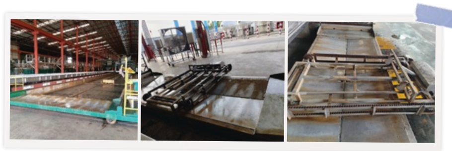
Electric Rubber Drying Trolley and Oven Trolley Pusher
